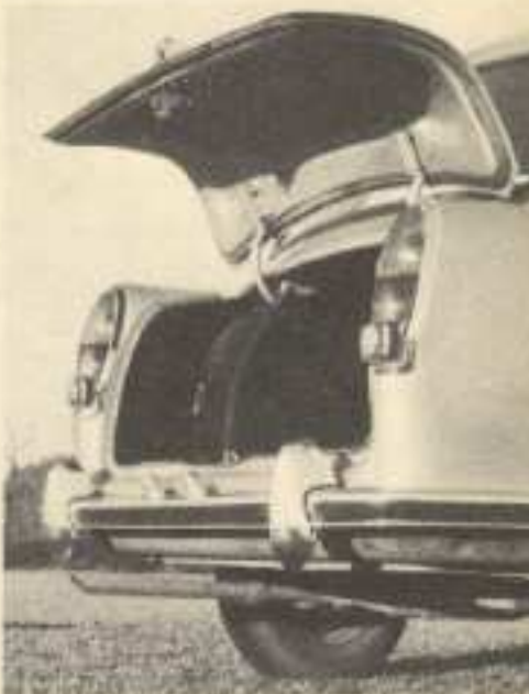
The bigger luggage trunk adds a bulge and 8½ in. of length to the car, but gives 8 cu. ft. carrying capacity. The lid rises upward to give clear access.
