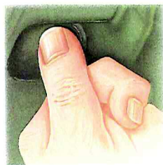
Remove the sparkplug from the timing cylinder and check with a thumb for rising air pressure as the piston comes up to TDC.
