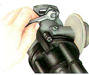
A distributor mounted on the end of the camshaft (in an overhead-camshaft design) is held by two or three bolts or studs in a slotted flange.
